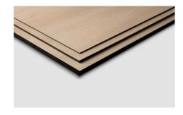
EGGER Compact Laminates black core are compact laminates according to EN 438-4, respectively EN 438-8 with a black core. They have a multilayer structure and consist of melamine resin impregnated decorative paper as surface layer and a fibrous and with curable resins impregnated core layer.
